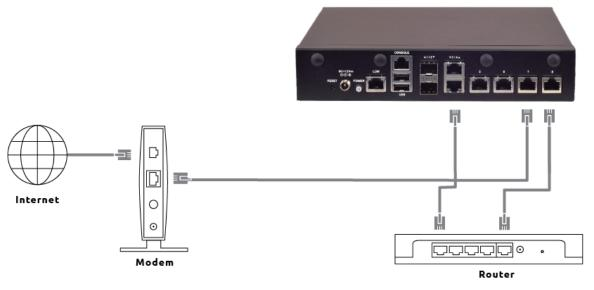
**5.** To configure and use the LiveWire Edge, connect Port 4 (eth3, MGMT) to the network.
